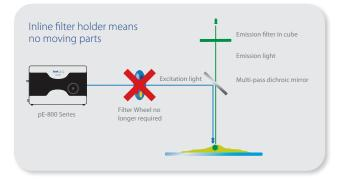
**pE-800**<sup>fura</sup> - Supercharged calcium imaging with lightning-fast,
