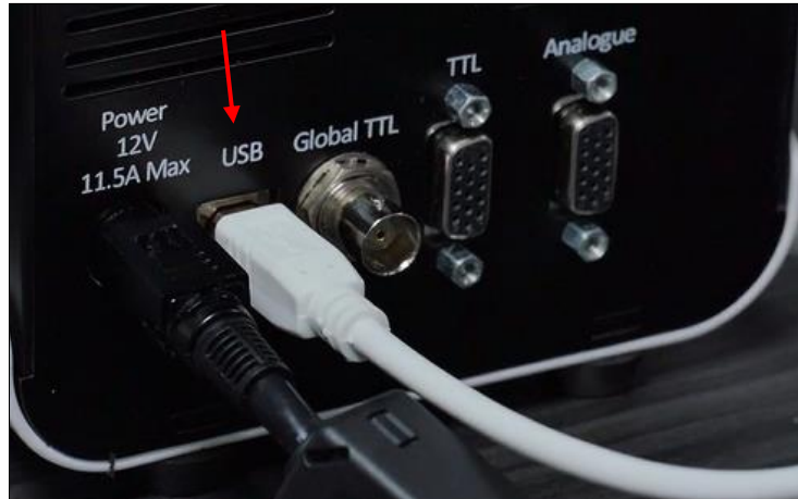
Figure 3: Connect the Illumination System to the PC via USB cable
