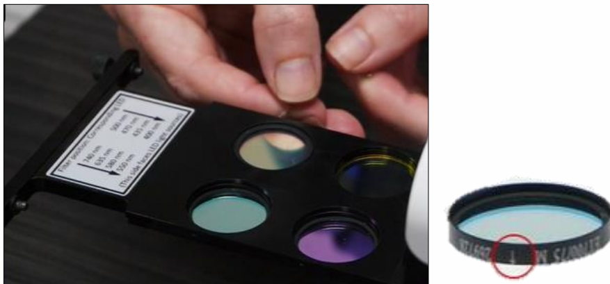
Figure 1: Installing excitation filters directly into the pE-800 Series and securing with grub screws
