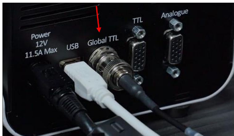
Figure 4: Directly connect camera and Light Source, inserting trigger cable into 'Global TTL' port
