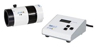
For IR-DIC, the pT-100 770 nm model is ideal and can be synchronised with the reflected light source with its TTL input.
