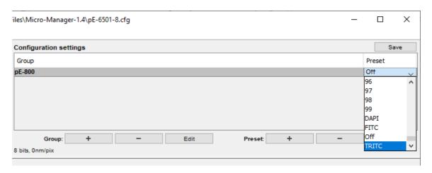
As the pE-6501-8 gives digital on/ off the intensities for the three separate LEDs should be set on the LightBridge software that comes with the pE-800.
