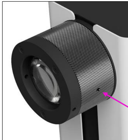
Figure 29: A pE-400 Series Direct Fit Light Source optical adjustment achieved by twisting the light output barrel. Grub screws (cyan arrow) must first be loosened.
