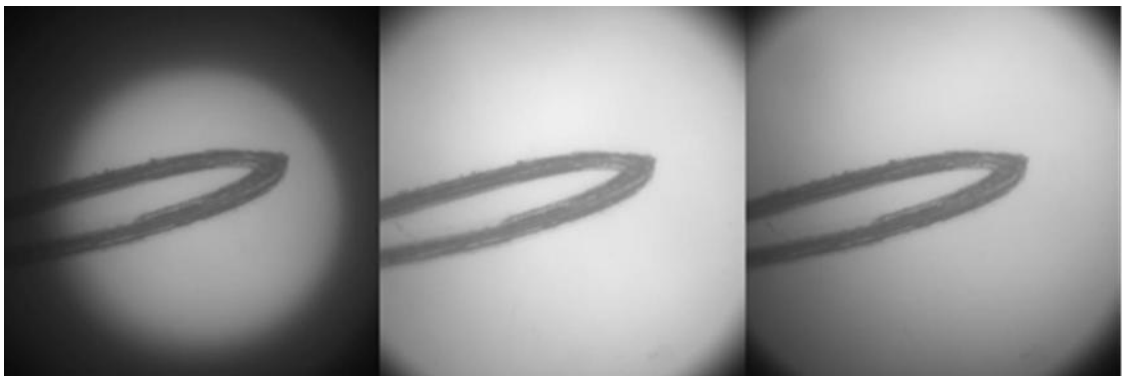
Figure 30: (From left to right) An underfilled sample plane (focus adjustments required), a central bright spot (focus adjustments required), most homogenous (optimal focus).
