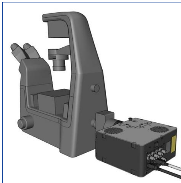
Figure 11: Figure 11 – A pE-400 max fitted to a microscope in a horizontal orientation
