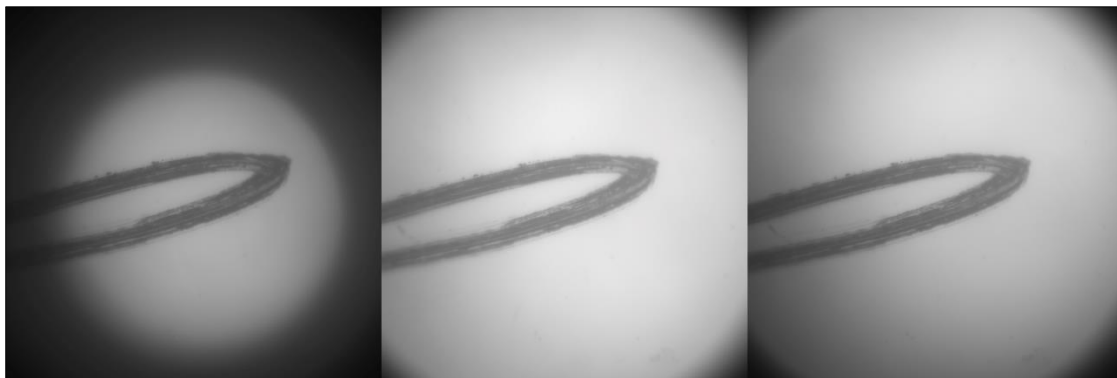
Figure 51 – (From left to right) An underfilled sample plane (focus adjustments required), a central bright spot (focus adjustments required), most homogenous (optimal focus).
