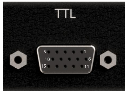
Figure 9: Physical position of TTL channels
