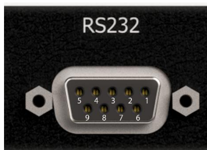
Figure 11: Physical position of RS-232 channels
