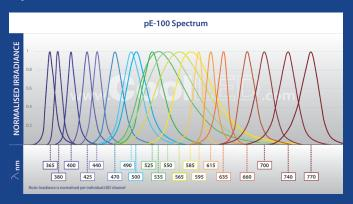
20 different LED wavelengths from the near-UV at 365 nm to the near-IR at 770 nm
