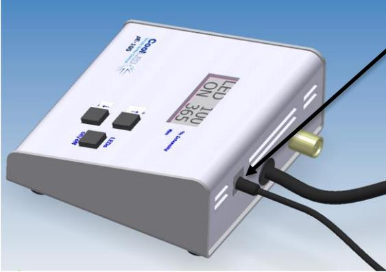
Insert the connector from the power supply into the Control Pod as shown.
