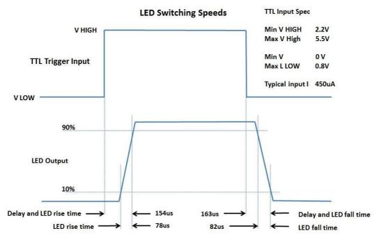
Note: Switching speeds vary slightly depending on LED wavelength and the intensity that is used.
