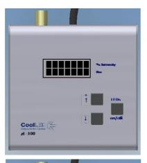
Upon switching on the Pod a chequered pattern shall appear on the display. If any button is pressed at this stage then you shall be taken through a setup sequence.
