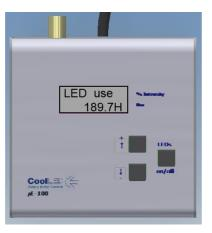
The system automatically records the total time that the LEDs are on.
