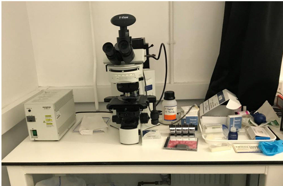
Figure 1. Olympus BX41 microscope with mercury-vapor lamp attached and power supply on the left.
