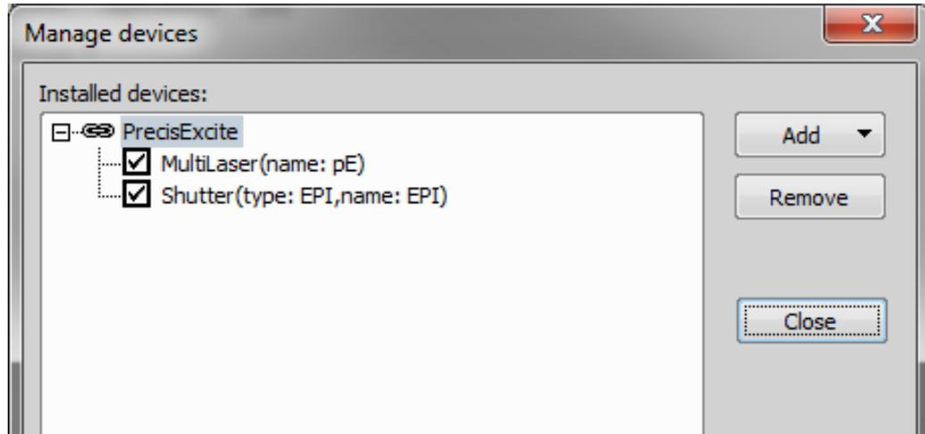
Figure 6: 'Manage Devices' window with 'precisExcite' connected
