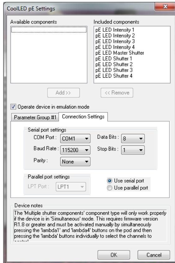
Figure 7: 'Connection Settings' for adjusting COM Port.
