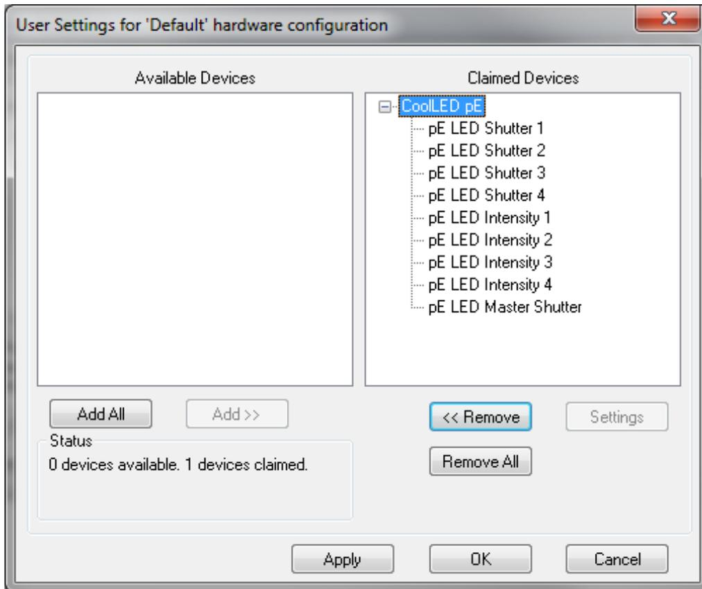
Figure 9: CoolLED pE Installed and 'claimed' in MetaMorph
