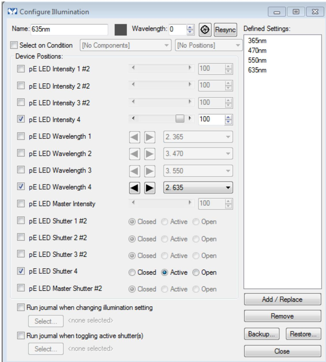
Figure 15: 'Configure Illumination' Window with several 'Defined Settings'
