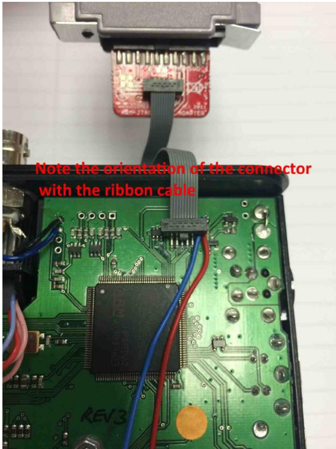
Figure 15. Main processor connection.
