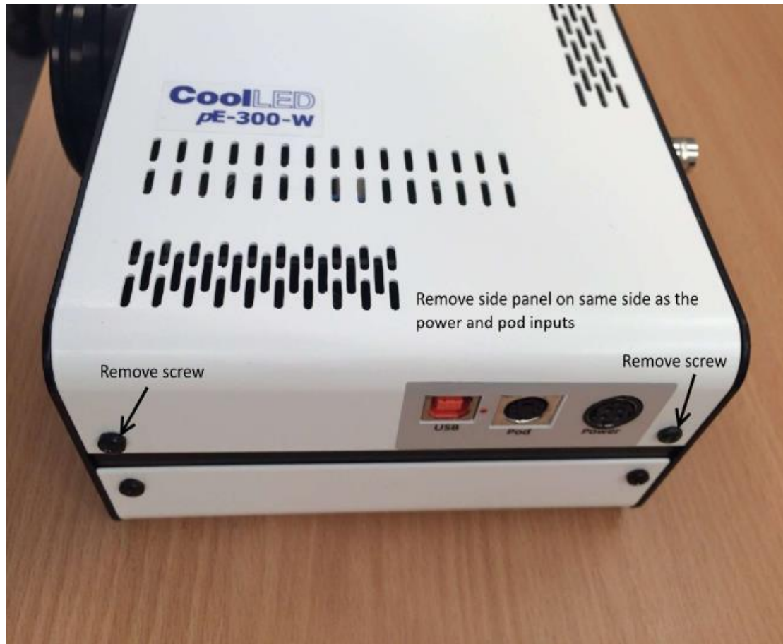
Figure 13: Side panel showing two of the four screws that need to be removed.
