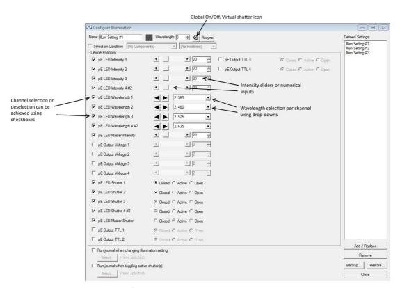
Individual channel control for intensity, channel and shuttering
