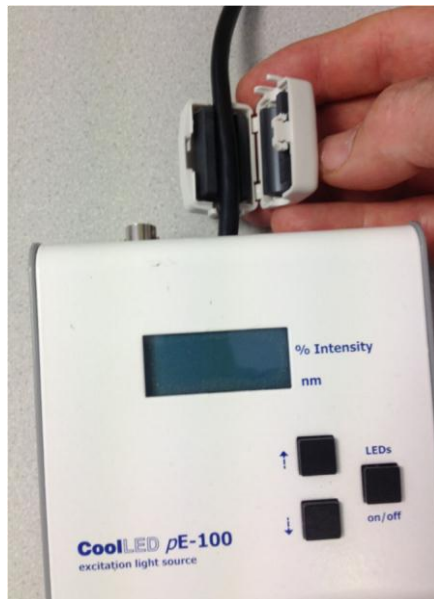
Place split core ferrite around
