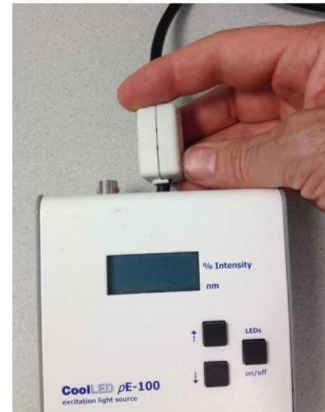
Ensure 2 halves are clipped together cable close to the pod
